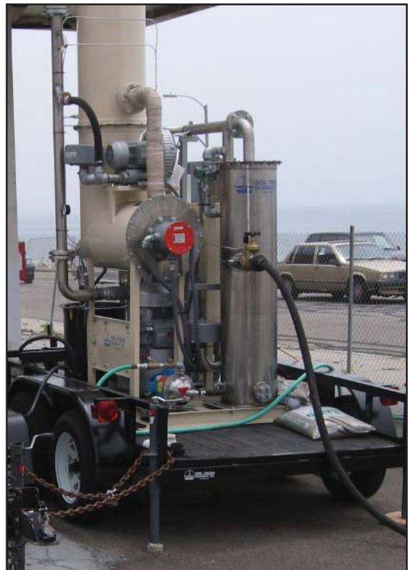
Soil-Therm Micro-ELECTRIC system with powerful Hi-Vacuum SVE Blower and Variable Frequency Drive for complete flow & vacuum range control to 14" Hg. Mounted onto a small 5'x10' dual axle trailer with room for Liquid GAC vessels.
